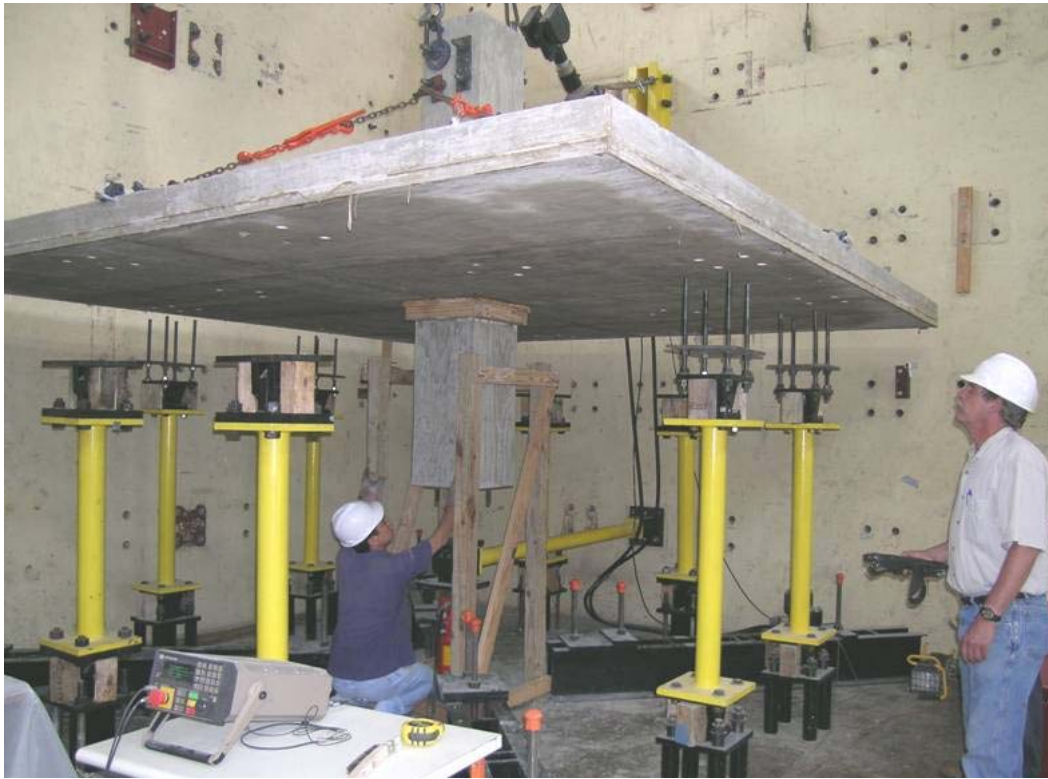
Figure 3.25 Installation of a test specimen
