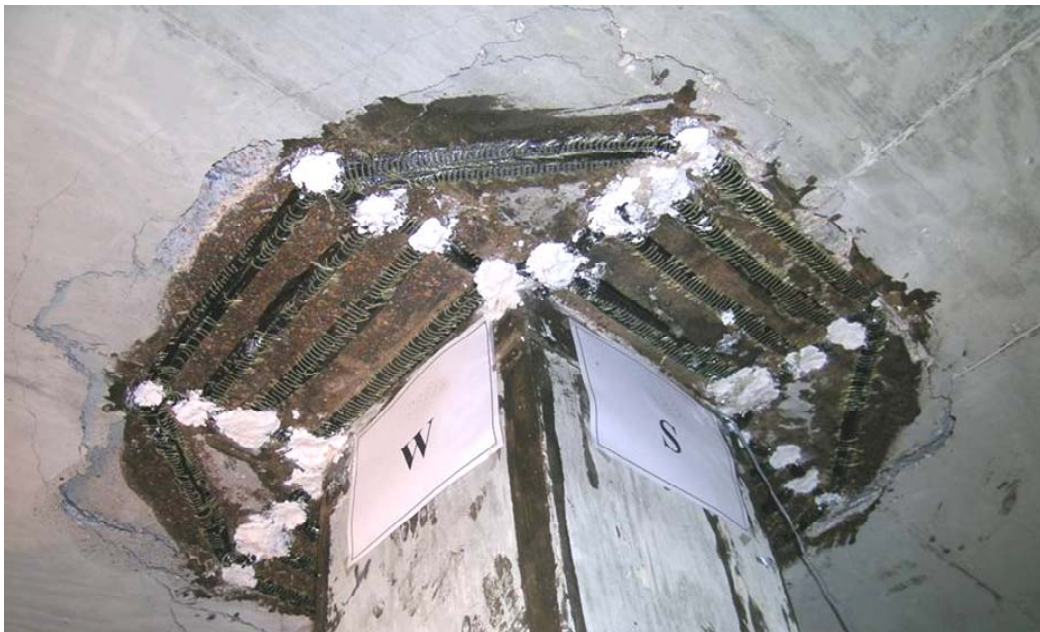
Figure 4.34 Failure surfaces of LRstG0.5
