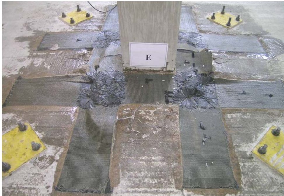
Figure 4.44 Top view of failure surface of LRshG0.5
