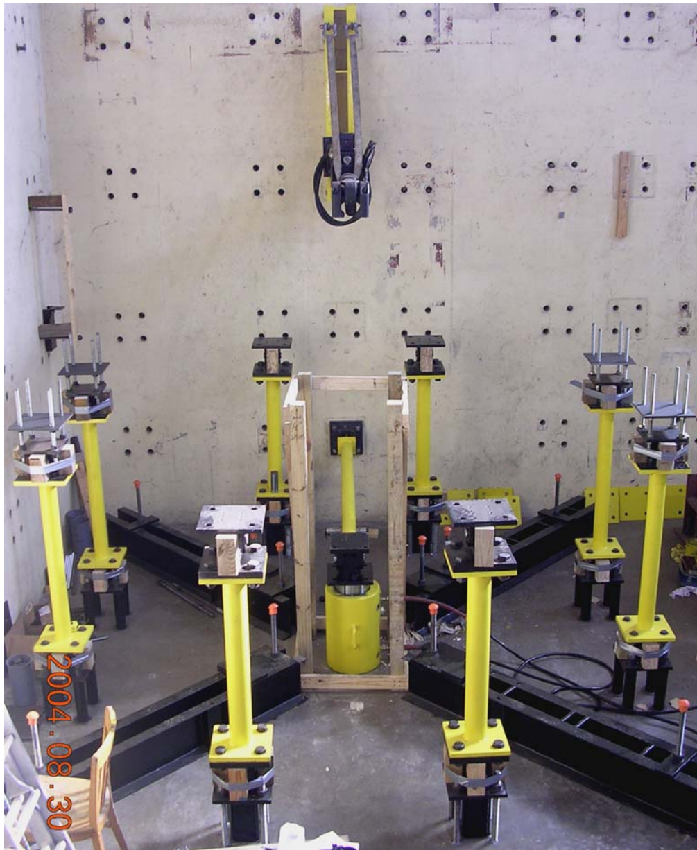
Figure 3.24 Position of vertical struts: simulated seismic test
