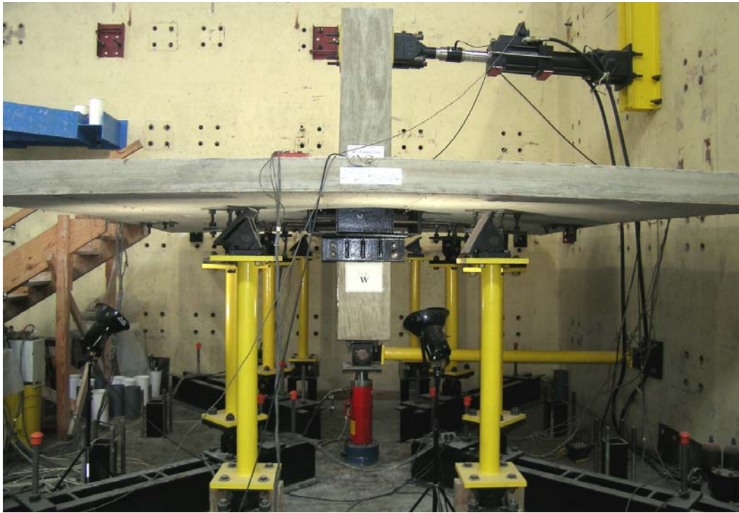
Figure 4.14 Significant vertical deflection at failure of RcG0.5
