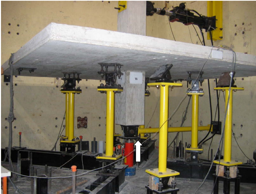
Figure 3.19 Test setup: Punching shear test
