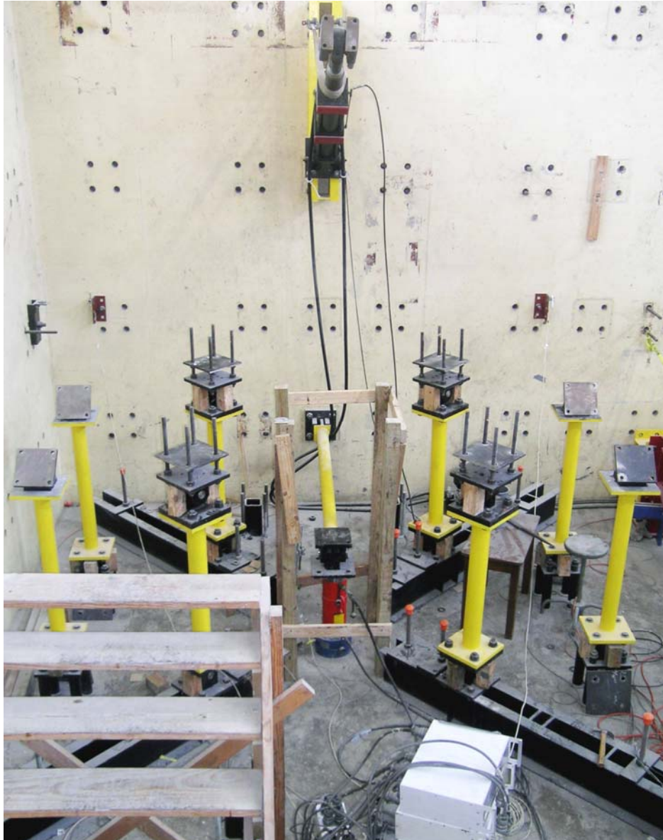
Figure 3.26 Position of vertical struts: punching shear test
